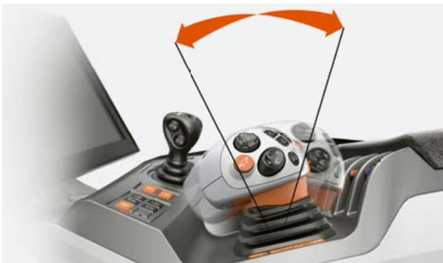
Progressieve bediening dankzij de CMATIC continue variabele transmissie technologie
