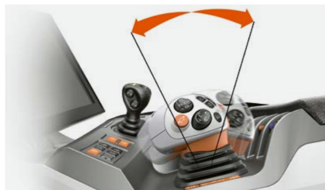
Progressieve bediening dankzij de CMATIC continue variabele transmissie technologie.
